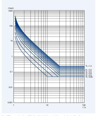
Note) If the operation time of the time-limited characteristic curve is shorter than the instantaneous operation, it is based on the instantaneous operation time.
