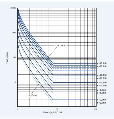
• Apply: THR(49) • HOT:  $t = \tau_h \cdot I_n \frac{I^2 - I_P^2}{I^2 - (k \cdot I_B)^2}$   $\tau_h = 2.0 \sim 60.0 \text{min}$ • COLD:  $t = \tau_c \cdot I_n \frac{I^2}{I^2 - (k \cdot I_B)^2}$   $\tau_c = 2.0 \sim 60.0 \text{min}$   $\begin{pmatrix} I_P = 0.5 \\ k = 1 \\ I_B = 1 \end{pmatrix}$ • k = SF
