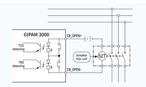
\* Terminal between the CB\_OPEN contactors may always have a resistance of around 200 k $\Omega$ , which may not operate normally when used for any purpose other than TRIP.
