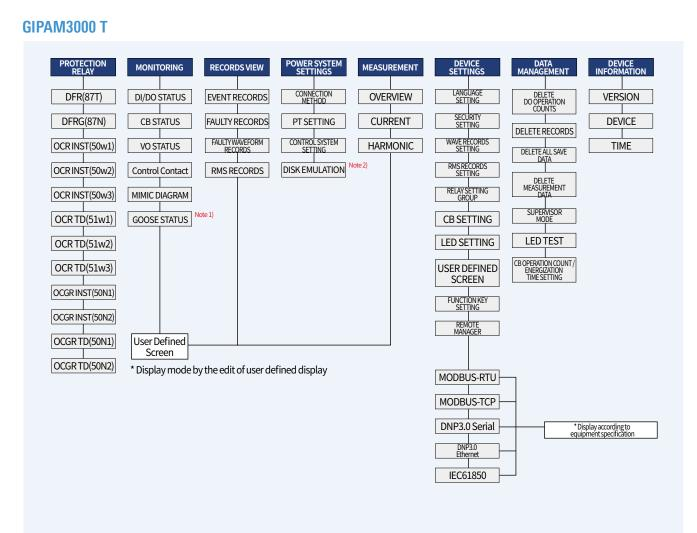
Note) 1. GOOSE reception status function: Refers to the function of displaying the reception status of the GOOSE message subscribed to in IEC 61850 communication.
